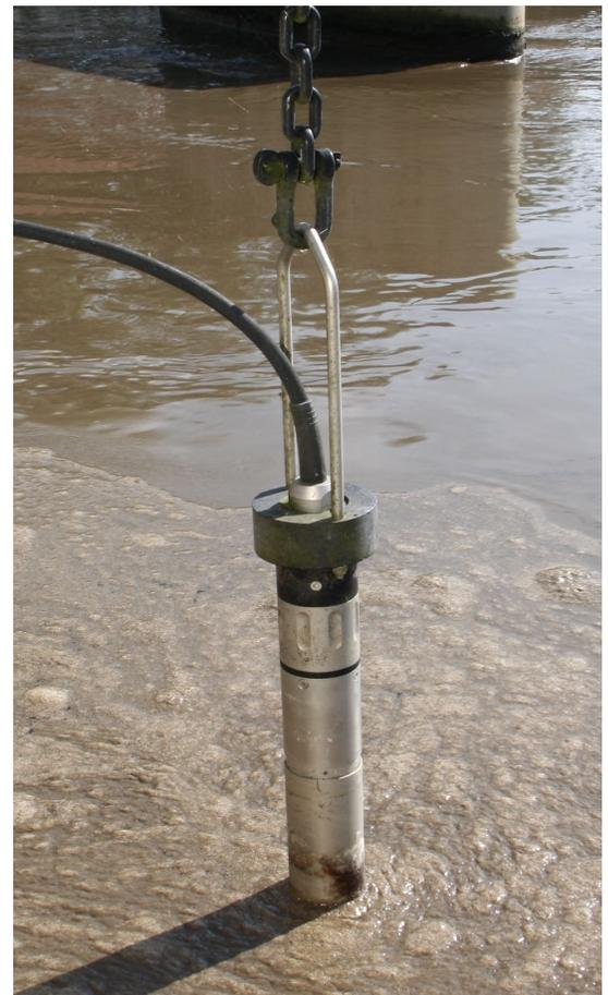
YSI IQ SensorNet ISE probe installed in anoxic zone of biological tank
